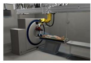
A high-mobility industrial robot by the name of Virtobot records the contours of a cadaver under examination. Using computed tomography at the same time, forensic doctors are provided with a three-dimensional image and can conserve corpses digitally.
